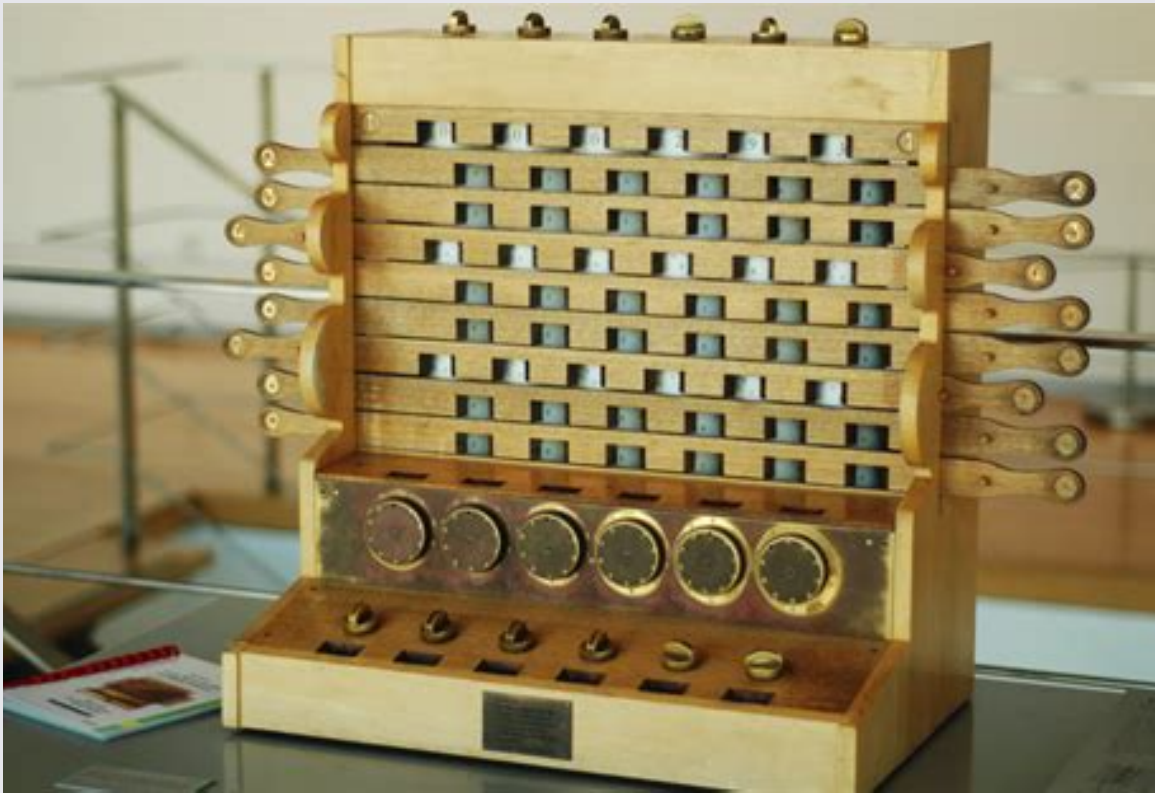
Figure 5.7 Wilhelm Schickard mechanical calculator (reconstruction)
